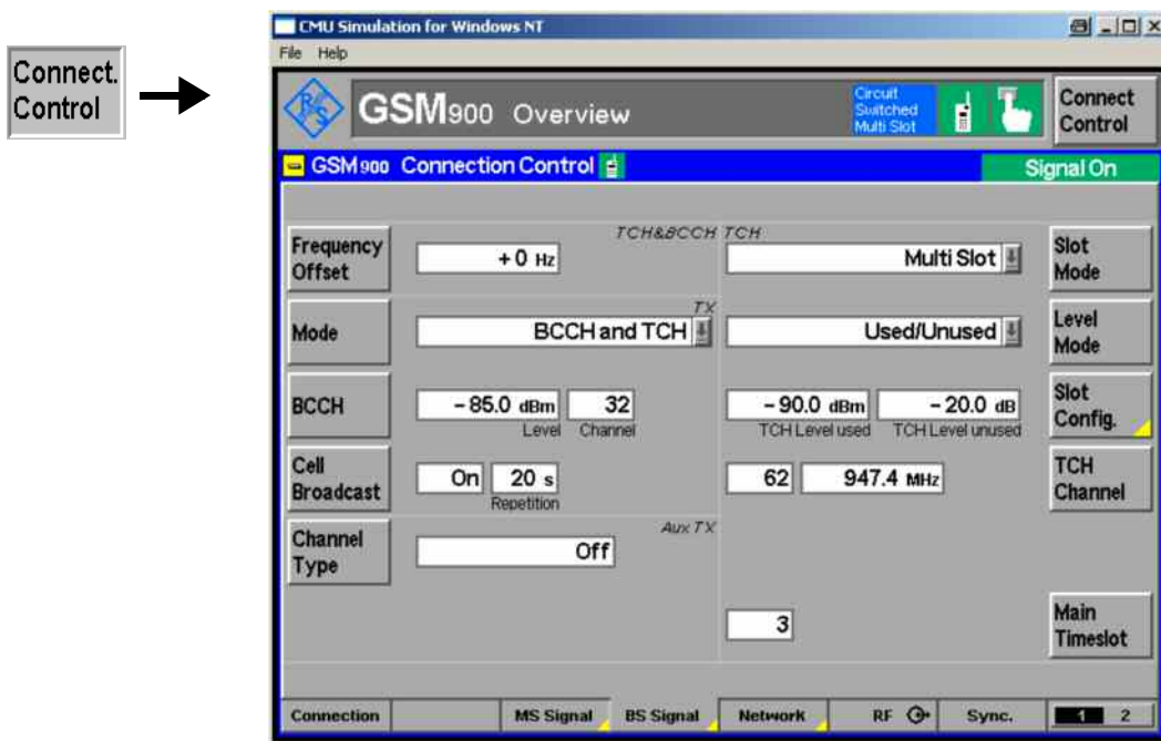
Fig. 4-107 Connection Control – BS Signal (panel, multislot)
